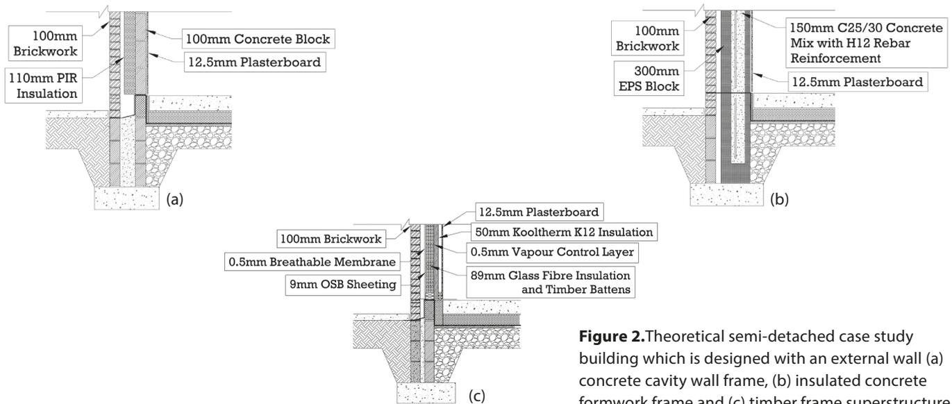
**Figure 2.** Theoretical semi-detached case study building which is designed with an external wall (a) concrete cavity wall frame, (b) insulated concrete formwork frame and (c) timber frame superstructure.
