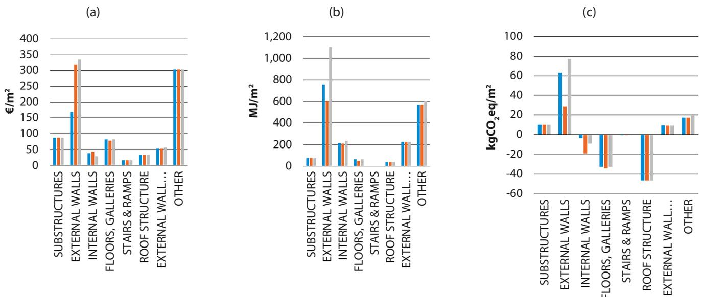
**Figure 3.** Life cycle (a) cost, (b) non-renewable energy and (c) GHG balance of the building elements in the superstructure designs. Blue = traditional; Orange = timber; Grey = ICF
