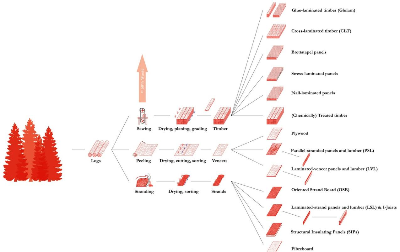
Figure 11 The main processing chains for timber products used in construction by Fleming (Ramage et al 2017)
