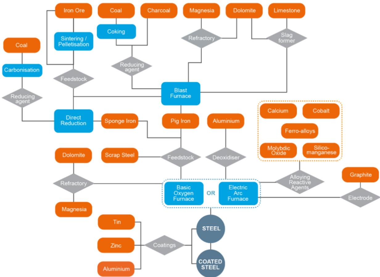
Figure 23 Simplified steel industry supply chain (World Steel Association, 2019)
