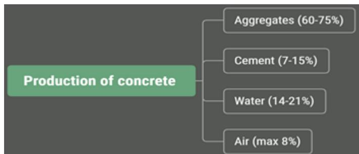
Figure 16 Average proportions of raw materials in concrete mix
