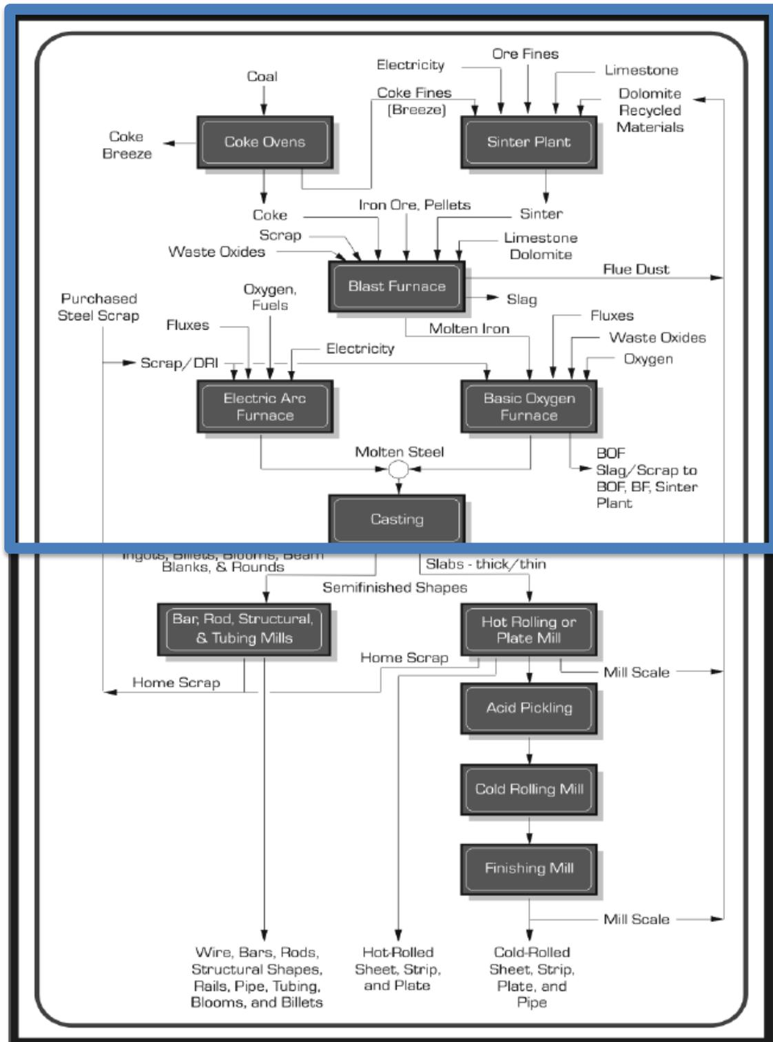
Figure 22 Process flow for steel making (Adapted by ITP Steel: Steel Industry Technology Roadmap, 2001<sup>4</sup>)
