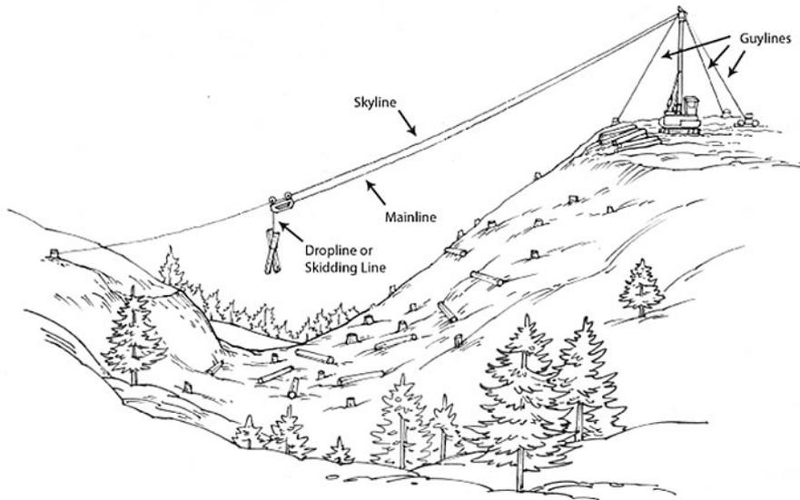
Figure 8: Cableyarding in steep terrain (Source: FED US)
