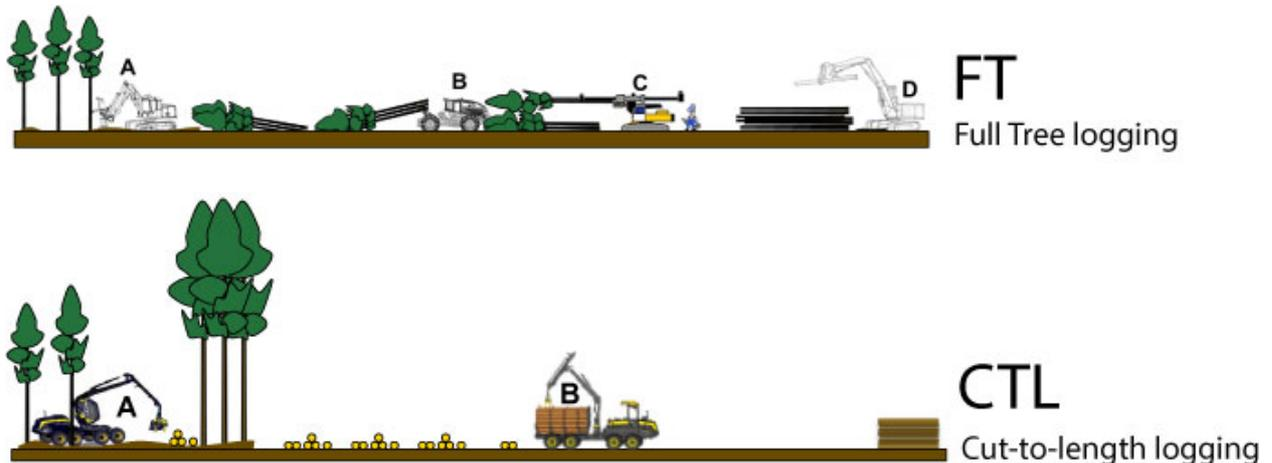
Figure 7: Cut-to-length versus tree length / full tree method (Source: PNG Biomass)
